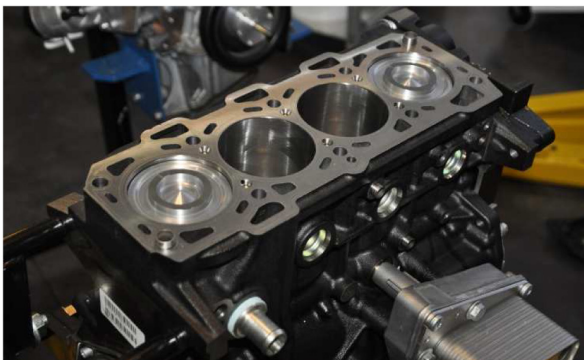
Figure 2. The 2-zone piston bowl geometry in CAD (top) and installed in the multi-cylinder GM 1.9L engine (bottom).
