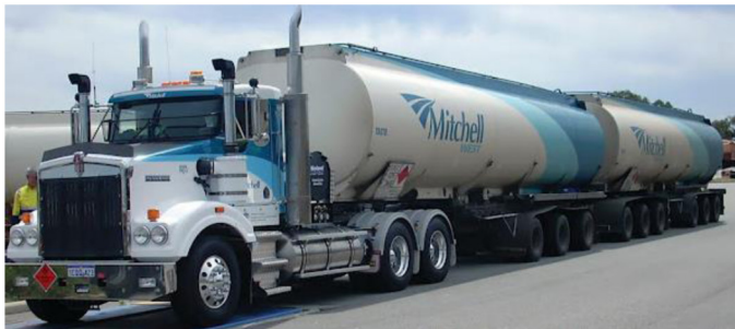
Figure 1. KW T408 SARE with a B-double trailer configuration powered by a 15 L HPDI engine in service in Australia
