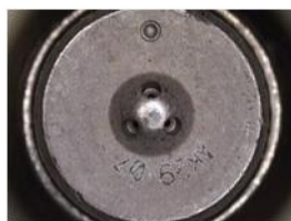
Figure 1. The purpose-built GDi seat design with 3 identical nozzles at uniform 120° circumferential spacing
