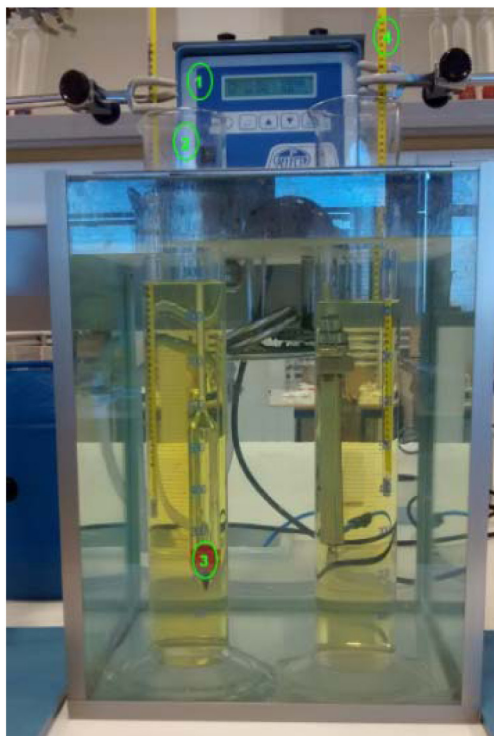
Figure 1. Setup for the measurement of density at atmospheric pressure. The image shows the different equipment used in the facility: 1) temperature regulator; 2) diesel specimen inside a test tube; 3) hydrometer; 4) thermometer.
