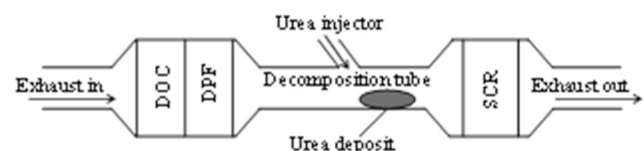
Figure 1. Schematic diagram of DEF-SCR aftertreatment system. DOC- diesel oxidation catalyst, DPF- diesel particulate filter, SCR-selective catalytic reduction
