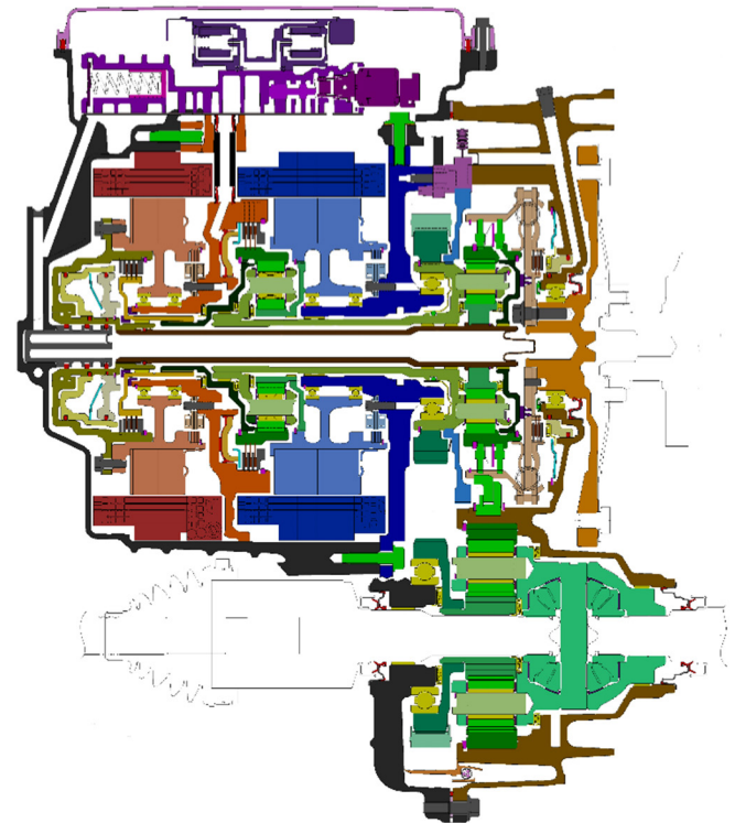
Figure 6. Voltec Drive Unit Cross-section
