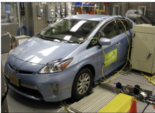
Figure 2. Toyota Prius Plug-in Hybrid Electric Vehicle loaded on a dynamometer in APRF
