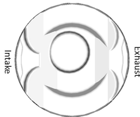
Figure 4. 12.5:1 CR piston topology.
