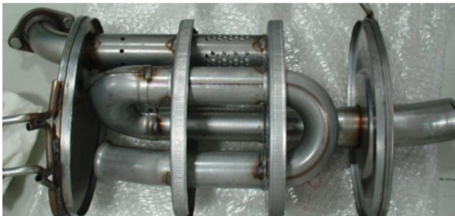
Figure 3. Internal structure of muffler
