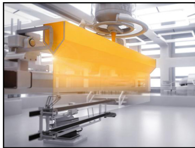
Figure 1. A schematic of the fusion draw process.
