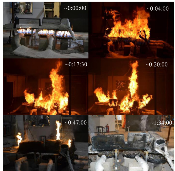
Figure 4. HRR test images: initial burner startup (top left); initial peak HRR (~550 kW) around 4:00 (top right); peak HRR (~700 kW) around 17:30 (center left); burners off around 20:00 (center right); small flames from battery vents around 47:00 (bottom left); and visible flames extinguished around 1:34:00 (bottom right).
