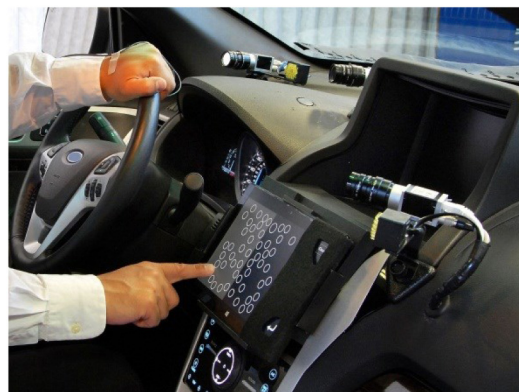
Figure 3. Microsoft surface for SuRT with mounts in the instrumented vehicle
