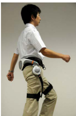
Figure 1. Honda Stride Management Assist (SMA) device.
