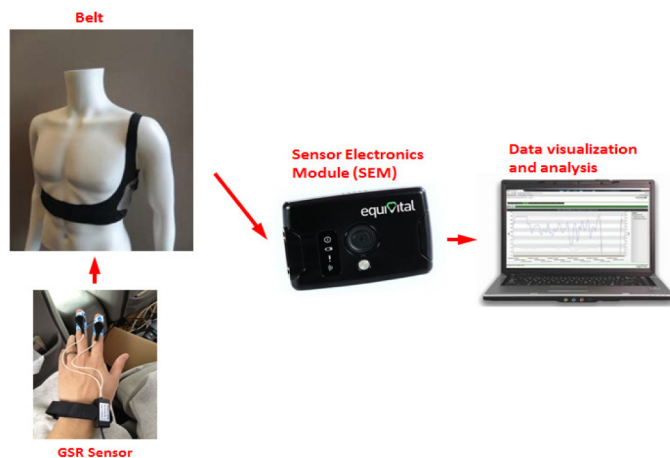
Figure 2. Physiological signal acquisition equipment.
