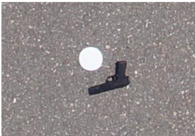
Figure 3. Image of a circular plastic target next to a handgun taken by a 24-megapixel camera at 20 meters flying height.
