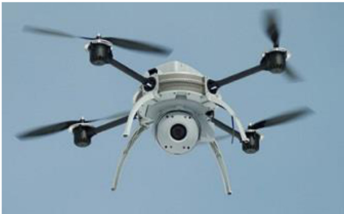
Figure 6. Aeryon Scout with 4-megapixel integrated, stabilized camera. Manufactured by Aeryon Labs, Inc.
