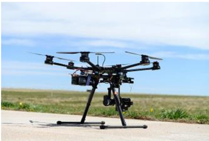
Figure 7. DJI S800 with Zenmuse brushless gimbal and Sony NEX-7 24-megapixel camera with 24 mm Zeiss lens. Manufactured by DJI.
