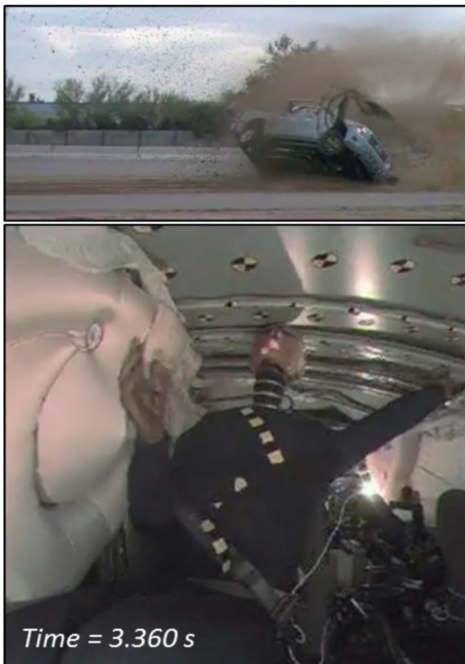
Figure 17. Exterior pickup orientation (top) and passenger ATD position (bottom) after movement of seatbelt relative to ATD shoulder (roll angle = 316°, and roll rate = 535°/s).
