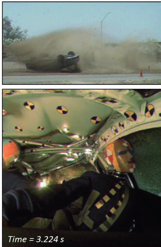
Figure 7. Exterior view of sedan position (top) and interior driver ATD position (bottom) that corresponds to neck loading event during the first roll (roll angle = 190°, roll rate = 404°/s).
