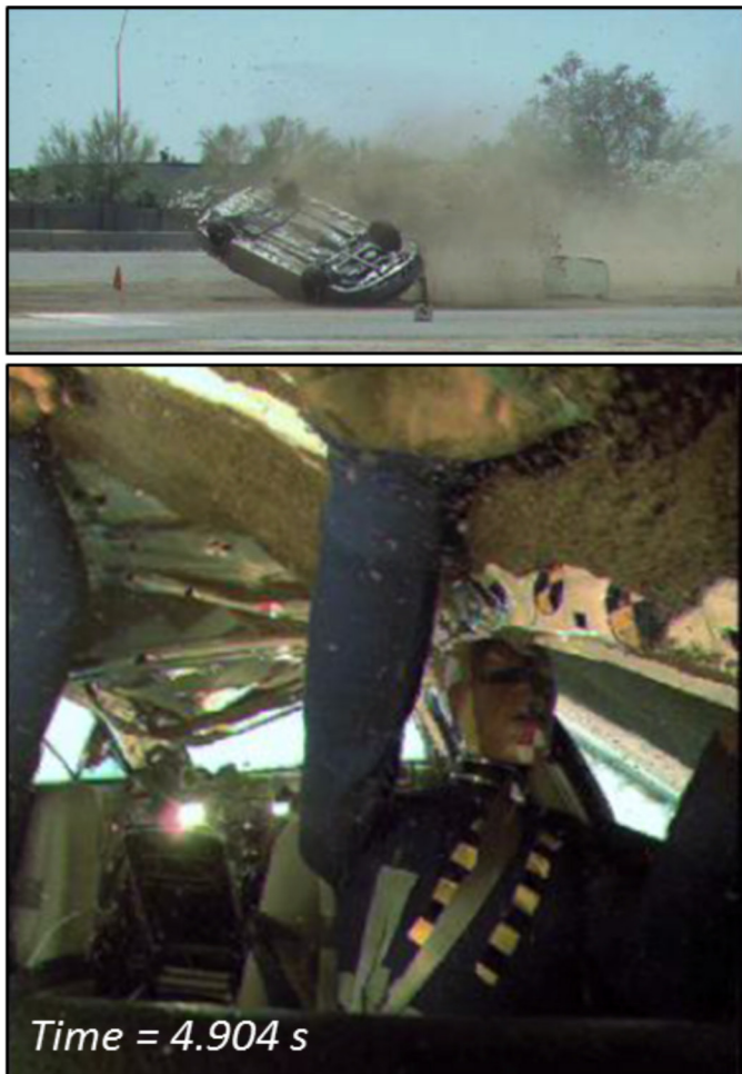
Figure 12. Exterior view of the sedan orientation (top) and interior view of the driver ATD position (bottom) that corresponds to the neck loading event during the third roll (roll angle = 720+212^\circ , roll rate = 315^\circ/\text{s} ).
