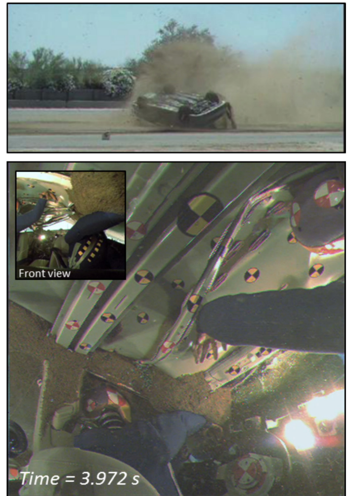
Figure 10. Exterior sedan orientation (top) and interior view of driver ATD position (bottom) that corresponds to neck loading event during the second roll (roll angle = 360+200^\circ , 461^\circ/s ).
