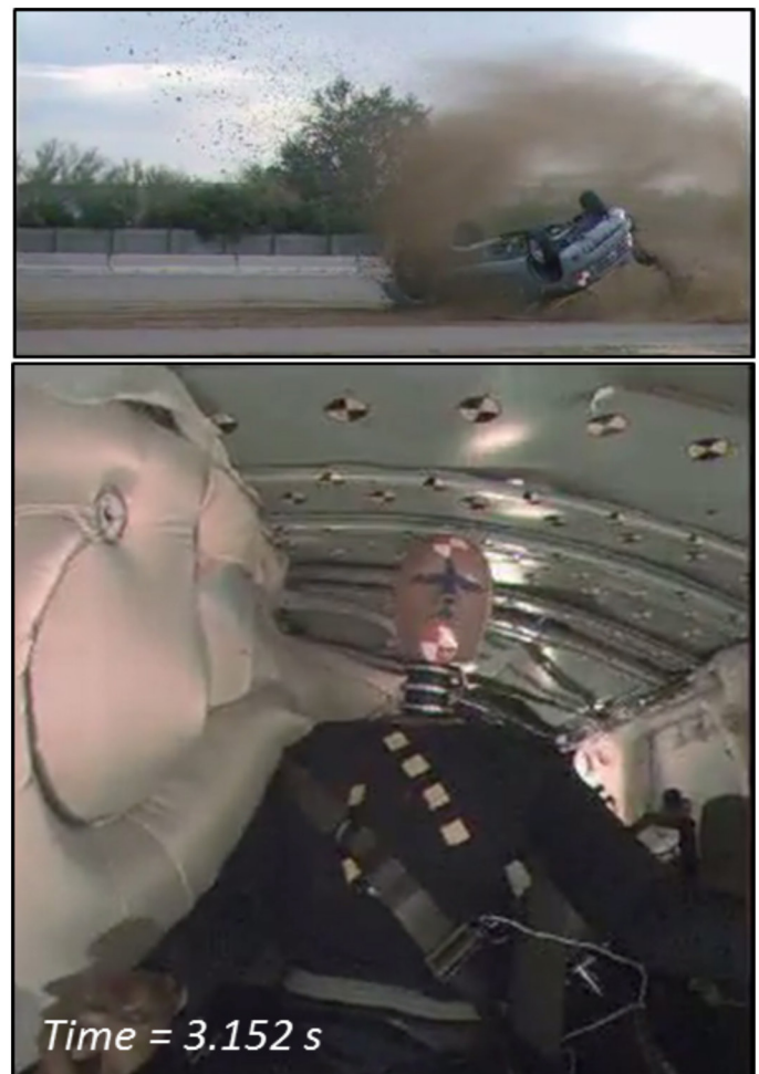
Figure 16. Exterior view of the pickup orientation (top) and onboard view of passenger ATD position (bottom) at time of vehicle-to-ground contact during first roll (roll angle = 207^\circ , and roll rate = 442^\circ/s ).
