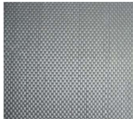
Figure 2. A bidirectionally woven glass fiber mat
