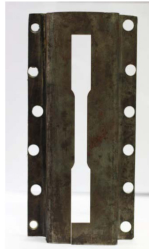
Figure 5. Formed double-hat face from which a tensile test coupon specimen is extracted
