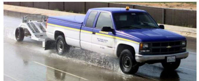
Figure 2. Braking Skid Trailer at Goodyear Proving Grounds, San Angelo, Texas
