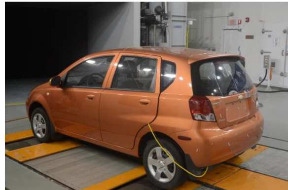
Figure 1. The test vehicle inside the climatic wind tunnel.
