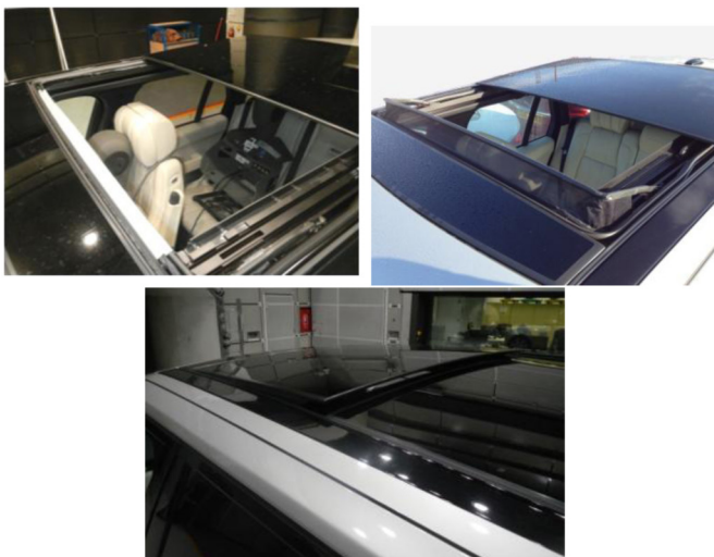
Figure 2. Range Rover sunroof configurations: (top left) deflector down; (top right) deflector up; (bottom) tilted sunroof
