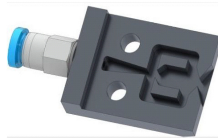
Figure 4. CAD model of the CNC machined main plate of the fluidic oscillator and pressure tube connector.
