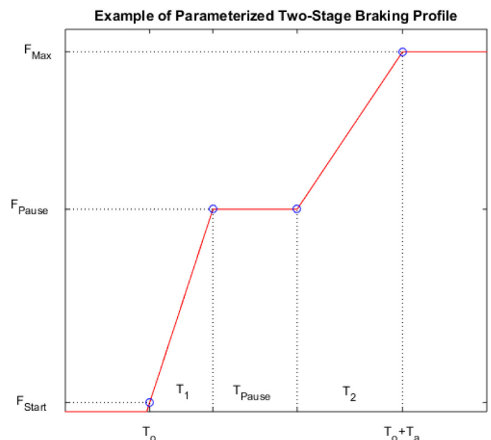
Figure 1. Example of a brake force application profile parameterized using a two-stage approach.
