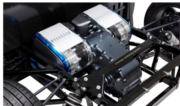
Figure 2. Rear powertrain of the xEV. There are the two air-cooled rear motors with the integrated inverters. The rear motors are connected to the wheels with the clutches. By disengaging them, the xEV can switch the 2WD and the 4WD modes while driving.
