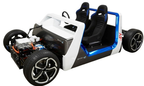
Figure 1. Powertrain concept car “EMIRAI 2 xEV”.
