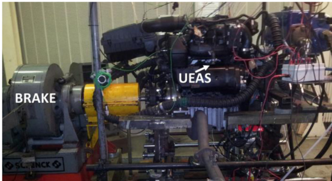
Figure 1. Sensors layout and engine test-cell installation
