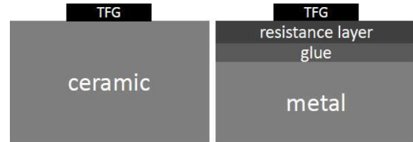
Figure 1. The two types of a TFG sensor: one directly painted on a ceramic (Macor®) substrate and one deposited on a resistance layer (Kapton®) that can be glued on any kind of surface.
