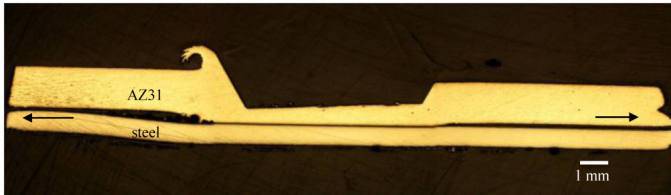
Figure 2. An optical micrograph of the cross section of an ultrasonic welded lap-shear specimen of magnesium and steel sheets.
