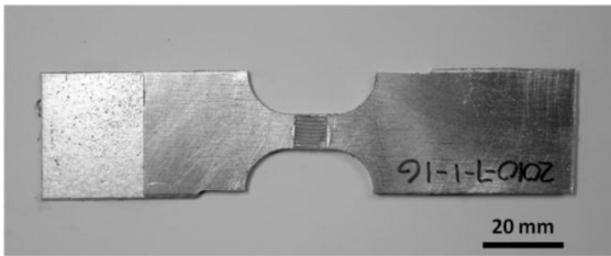
Figure 1. An ultrasonic spot welded lap-shear specimen of magnesium and steel sheets (a) before being machined and (b) after being machined into a dog-bone shape.
