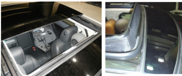
Figure 2. Sedan 1 tested sunroof configurations; (Left) deflector down; (right) mesh deflector up
