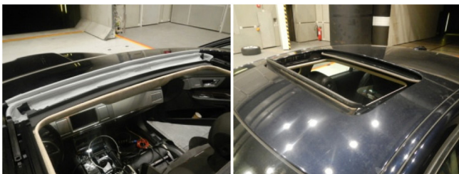
Figure 3. Sedan 2 tested sunroof configurations; (Left) deflector down; (right) mesh deflector up
