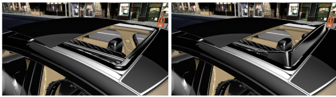
Figure 5. Simulated Sedan 1 configurations; (left) deflector down; (right) mesh deflector
