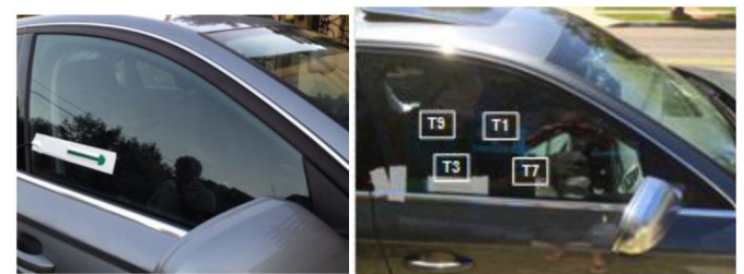
Figure 6. Stick-on/peel-off array applied to an automobile side glass (left) at four measurement locations (right)
