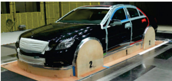
Figure 1. Example of vehicle setup with a skirt for blocking the underbody flow.
