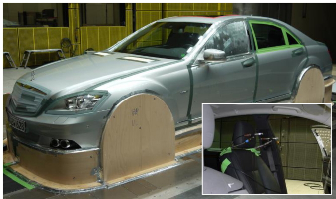
Figure 1. Mercedes-Benz S-class with blocked underbody flow and interior noise measurement at the driver's ears
