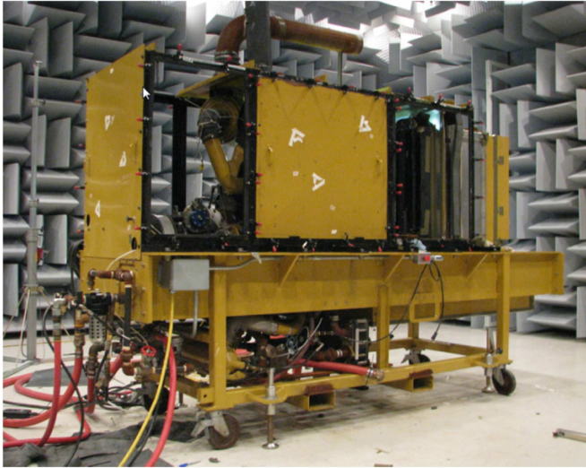
Figure 1. Engine test rig in a hemi-anechoic sound chamber
