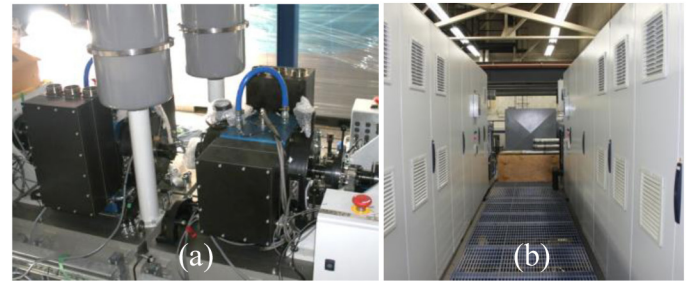
Figure 6. The drive stands (a) and the motor controllers (b) utilized in IPTMS. The engine emulator controls this hardware.
