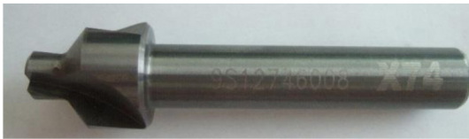
Figure 2. original countersinking tool - one for rough operation, another one for finishing operation
