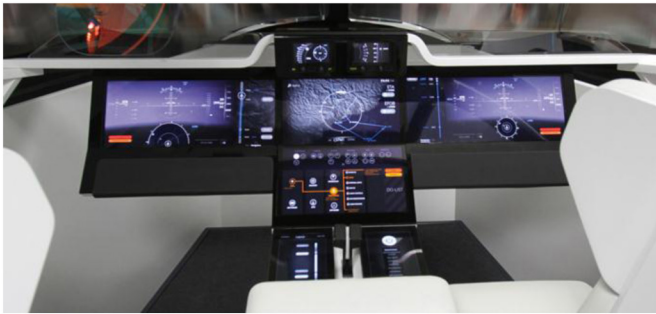
Figure 1. Avionics 2020 full touch screens cockpit (courtesy of Thales Avionics)
