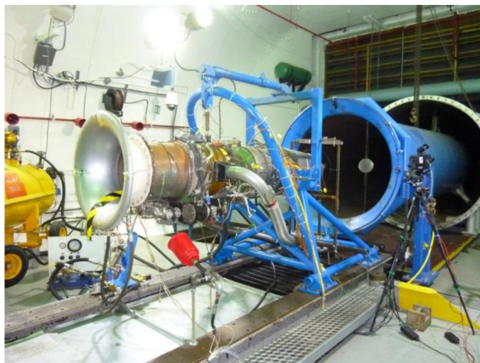
Figure 1. CF700-2D-2 turbofan engine core set up at NRC Canada.
