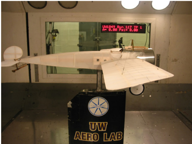
Figure 5. Fokker E.III in Kirsten Wind Tunnel, photo by University of Washington Aeronautical Lab.
