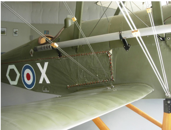
Figure 1. RAF SE5a wire bracing, photo by Scott Eberhardt.
