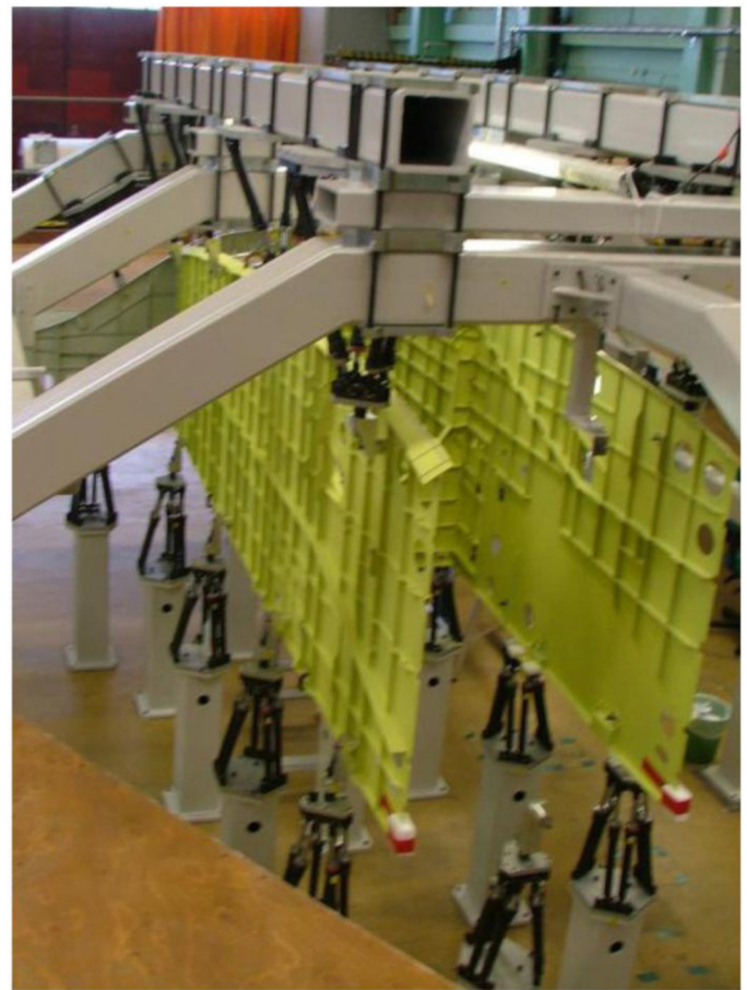
Figure 8. Industrial use of Hexapods and Boxjoint system configured for airframe assembly [18]
