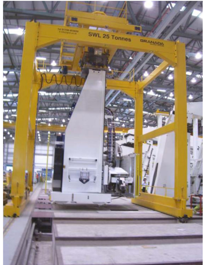
Figure 3. Automated drilling equipment is moved between wing fixtures [10]
