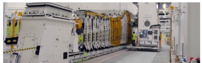
Figure 4. Wing assembly system with mobile automated drilling and bolting system [14], [15]
