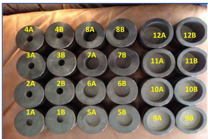
Figure 1. Photograph of Prototype Phenolic Pistons of Various Geometries (2 samples of each, labeled “A” and “B”)
