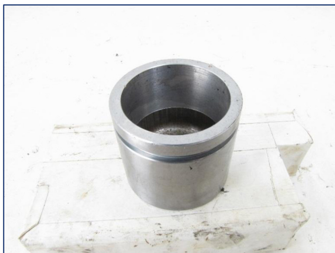
Figure 2. Photograph of Prototype Steel Piston (tight and loose specimens appear identical)
