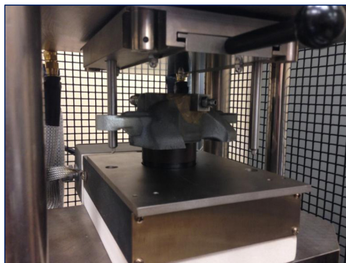
Figure 3. Piston Compression Test Wet Fixture
