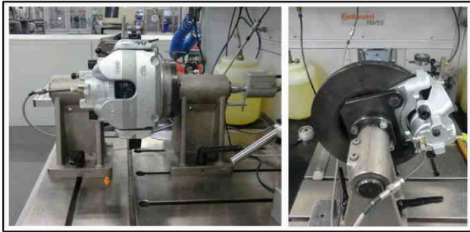
Figure 3. Drag torque measurement in the static test facility
