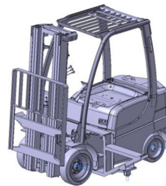
Figure 13. CAD representation of test truck geometry.
