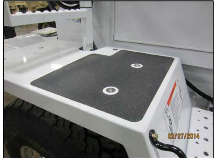
Figure 8. Example of slip resistant coating, 3M safety walk general purpose adhesive-backed applique installed on a front discharge cement mixer.
