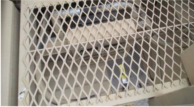
Figure 5. Example of expanded metal grate on US military vehicle.
