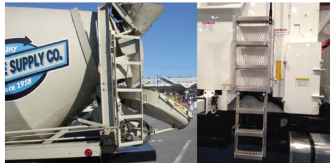
Figure 3. Examples of cab or body access step ladders employed on over the road and off highway vehicles.
