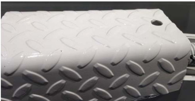
Figure 7. Example of rolled diamond plate steel in a cab access step application.
