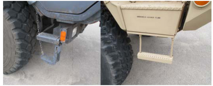
Figure 2. Examples of stirrup style access step utilized on US military vehicles.
