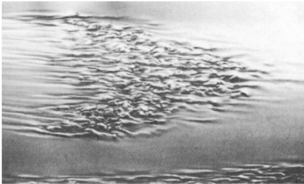
Figure 2.5. Photograph of turbulent spot in a transitional boundary layer, flow left to right [142].
