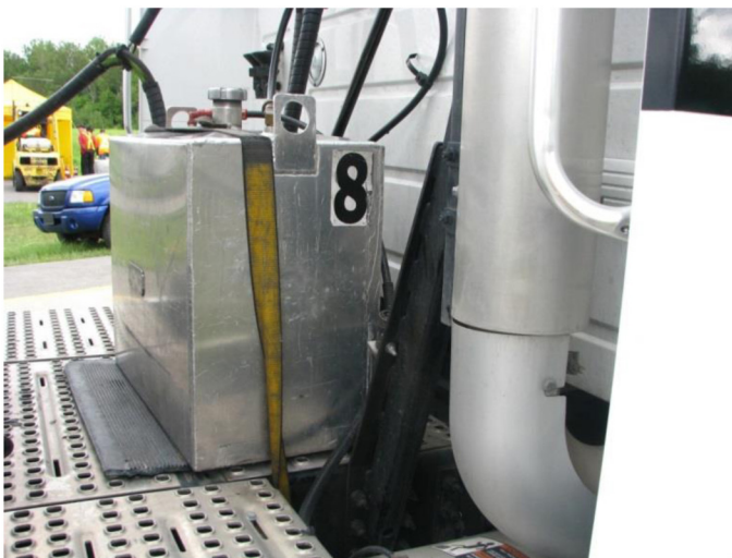
Figure 3. Installation of the portable fuel tanks
