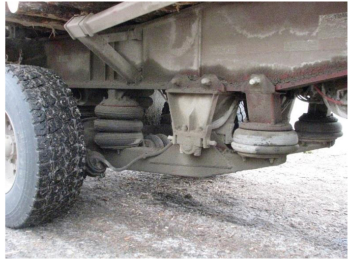
Figure 2. Air suspension of a lift axle on a forestry trailer
