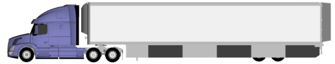
Figure 1. Photograph and side image of the study's baseline Volvo VNL670® with full side-skirt and boat-tail.
