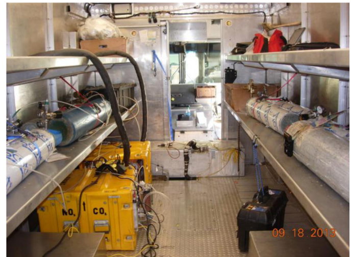
Figure 2. RAVEM system installed in the hybrid truck
