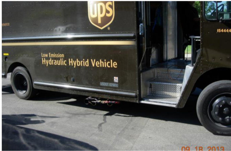
Figure 3. Isokinetic probe and sample line installed in the exhaust outlet of the hybrid vehicle
