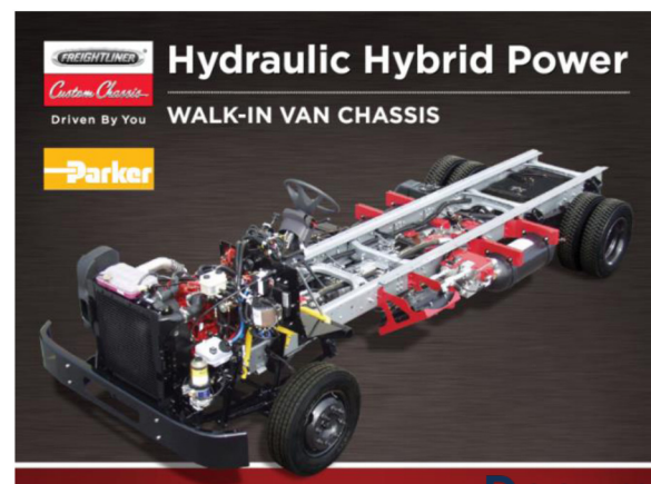
Figure 1. The FCCC / Parker Hannifin hydraulic hybrid walk-in chassis.
