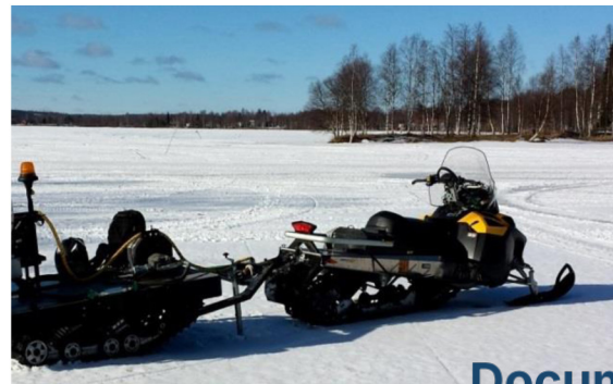
Figure 1. Test vehicle inclusive test trailer used to increase engine load
