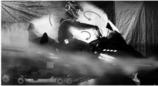
Figure 2. Using smoke to visualize external airflow in wind tunnel testing
