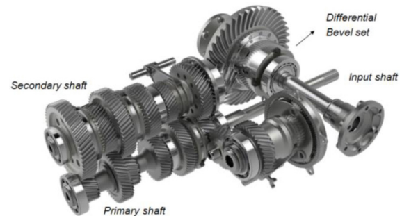
Figure 2. Three-dimensional view of the '6+2' hybrid electric drivetrain
