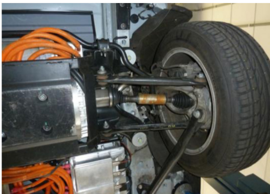
Figure 3. Rear axle drive elements
