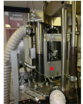
Figure 5. Hydro-pulse test rig - left: 1 rack, 2 load cell, 3 hydraulic cylinder, 4 bushing, 5 mounting / right: photo of test rig with heating chamber (red dot)
