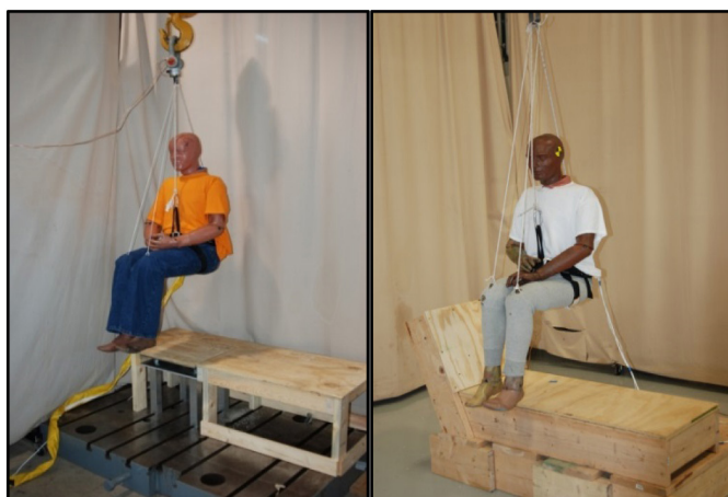
Figure 1. Photographs of ATDs and seat frames in the pre-drop orientation (from 20 inches) from Phase I (left) and Phase II (right).
